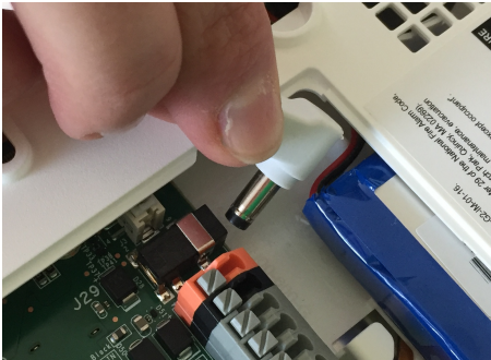
Plug in the power connector
