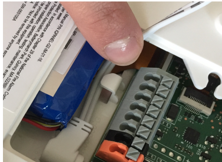
Route the wire behind the retainer clip
